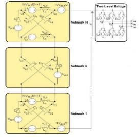
Figure 6.trapped inductor Z-source inverters
