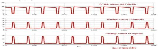
Fig.( 9c). Simulink dc-link and winding waveforms of Γ-Z-source inverter when in voltage-boost mode.
