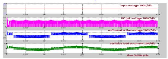
Fig.(9a) Simulink input, dc-link and output waveforms of  $\Gamma$ -Z-source inverter when in voltage-boost mode in R-LOAD
