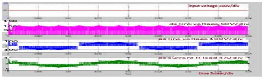
Fig. (10). Simulink input, dc-link and output waveforms of  $\Gamma$ -Z-source inverter when in voltage-buck mode.
