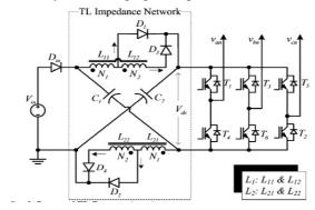
Figure 5.trapped inductor Z-source inverters
