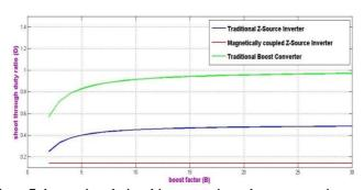
Figure 7. duty ratio relationship among impedance source inverters
